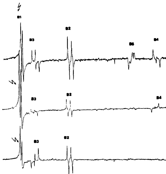
Figure 7. Single (bottom), double and triple (top) RELAY experiments using DANTE + CSSF technique (pulse sequence as shown in Fig. 8).
